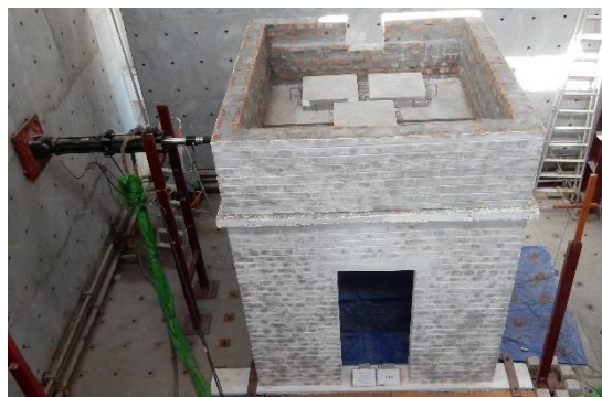
Fig.1. Test Setup for URM Building
