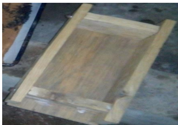
Fig. 2 Mould adopted for moulding of stabilized block
