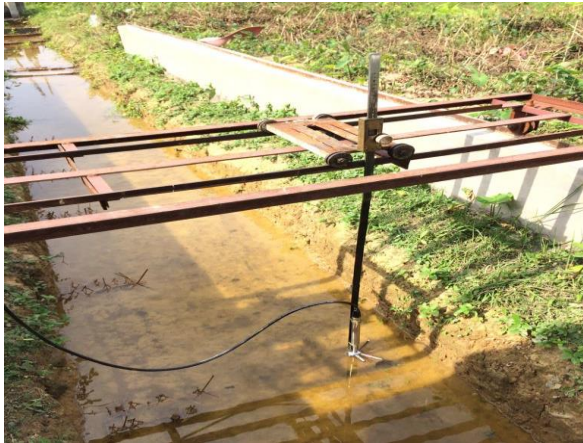
Fig 5: The ADV with probe installed inside the channel
