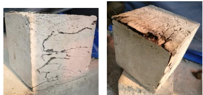
Fig 2: M20 Concrete Cube after failure
