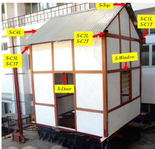
Fig. 6. Location of accelerometers in the specimen.
