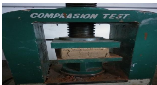
Fig. 3 Compression test on test block
