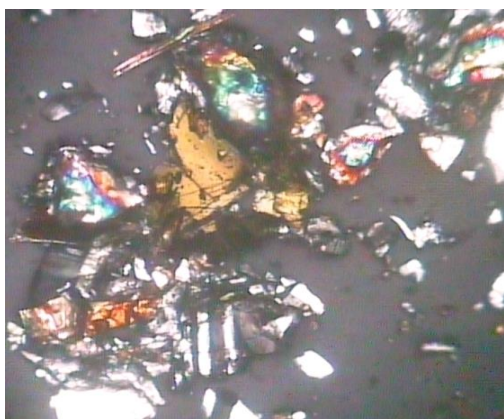
Fig. 2. Micro-photograph showing petrographic characteristics of quarry dust ( x 25)
