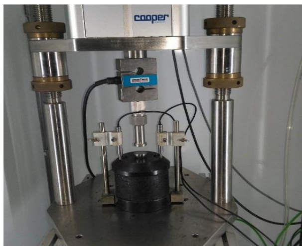
Fig. 1 The specimen is mounted in UTM for static creep test These tests are performed at 40°C in the
